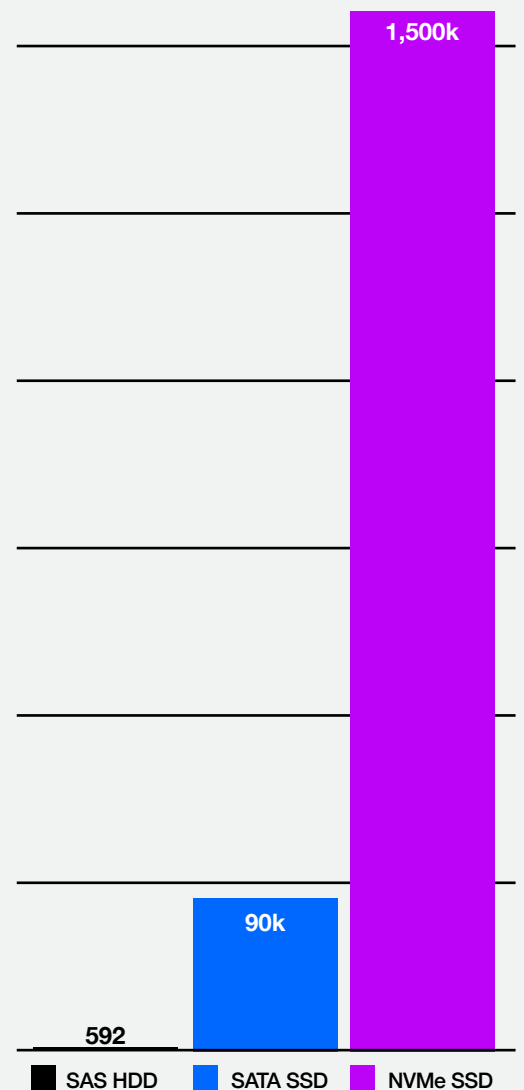
Figure 1: 4K random read IOPS for NVMe SSDs are 22x faster than SATA SSDs. 1
